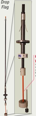
HIGHLY VISIBLE drop rod that signals when displacement limit has been exceeded
