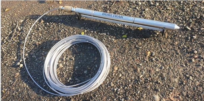
Boretrak2 probe with steel cable supplied for downhole deployments
